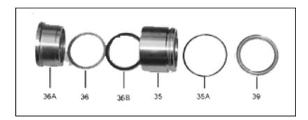
9. Lubricate weep seal (36). Place, weep seal (36), and pressure ring (36A) into the seal sleeve (35). Assemble the o-ring (35A) onto seal sleeve and lubricate.
